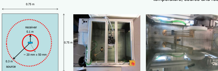
Fig. 1: The DBUS scanning system; top view (left and middle) and side view (right):
